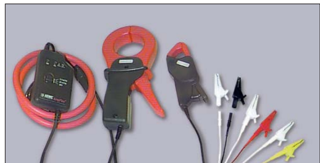
Voltage and current probes connect easily and never require an external power supply.
