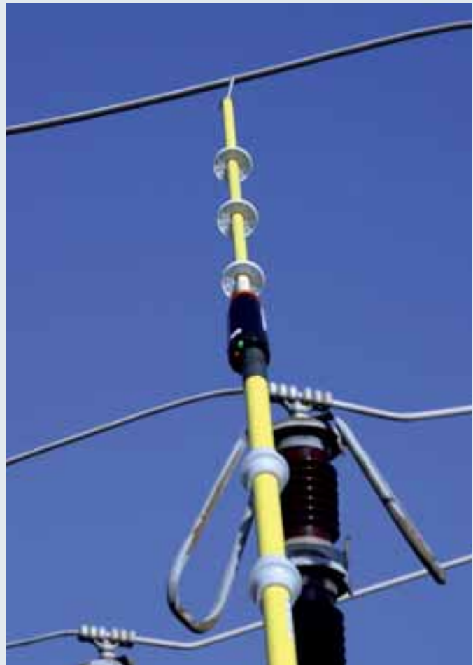
PHE III voltage detector used in an 110 kV outdoor installation.
