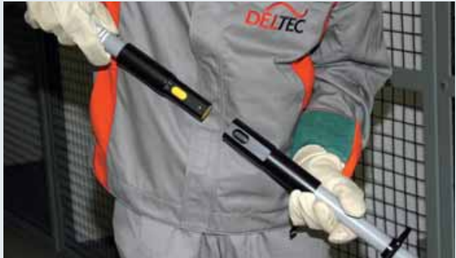
Plugging extension handle type HV STK into insulating rod type IS PHE STK.
