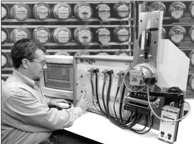
PHAZER Model T20 (for testing panel-mounted or bottom-connected meters) features external current and voltage output binding posts and a remote optical/control unit.
