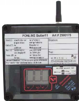
Option: Retrofit set type PONLINE-Butler11 with integrated IKI
