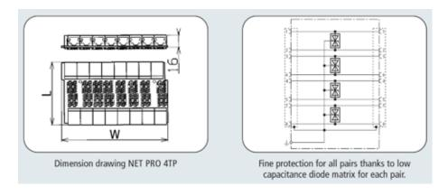
Fine protection board with 8 shielded ports for universal cablings (Class D). For universal use as protection for all 4 pairs (4 TP) is provided. To be installed into NET Protector 19" Enclosure and mounted into the distribution cabinet as a patch field or retrofitting unit.
