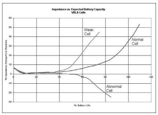
Figure 2. Impedance increases with battery age (and weakness).
