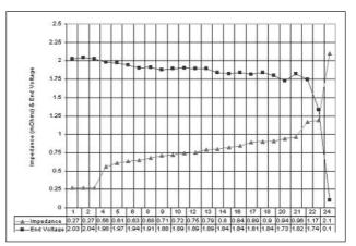
Figure 4. Ascending impedance compared to load test
