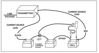
Figure 3. A typical test setup.
