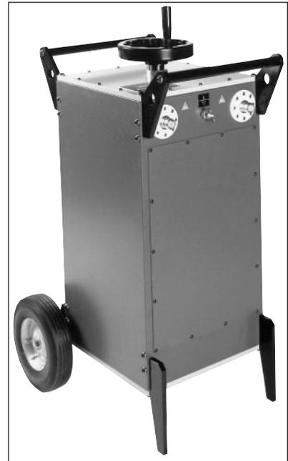
The optional Resonating Inductor expands the capacitance range of the DELTA 2000.
