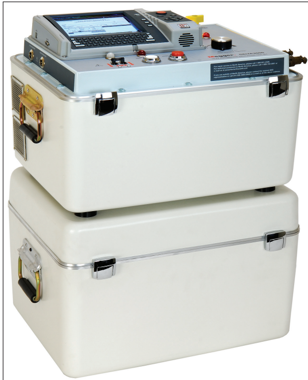
The DELTA3100, available in either 120 or 240 V ac/50 or 60 Hz, includes the control unit (top) and auxiliary module (bottom) containing HV amplifier and LV three-phase TTR circuitry.
